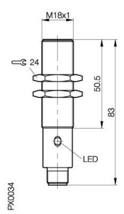
Inductive Sensors BES 516-326-S 4-C M18x1 x 83 normally-open Sn=5mm shielded
